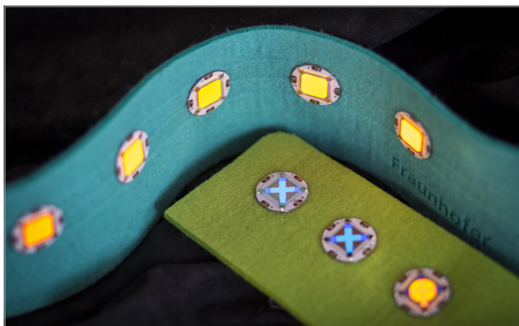
O-BUTTON, customer-specific OLED elements for textile integration
